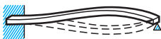
Figure 7.25 A beam built in at one end and simply supported at the other.
